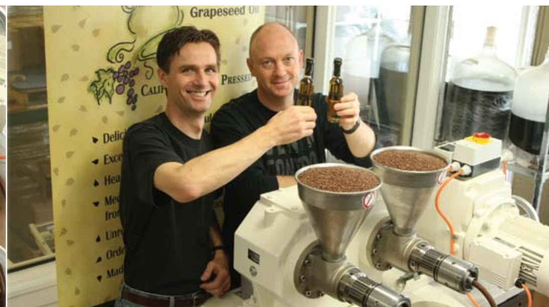
Opposite page: Valentin and Nanette show off a one-ton bag of prepared grape seeds. Below: Grape seeds being milled with the oil flowing into the saucers. The tube of brown “cake” comes out the front. Valentin toasts Dirk Skuras, Managing Director of IBG Monfort, maker of the oil press.
