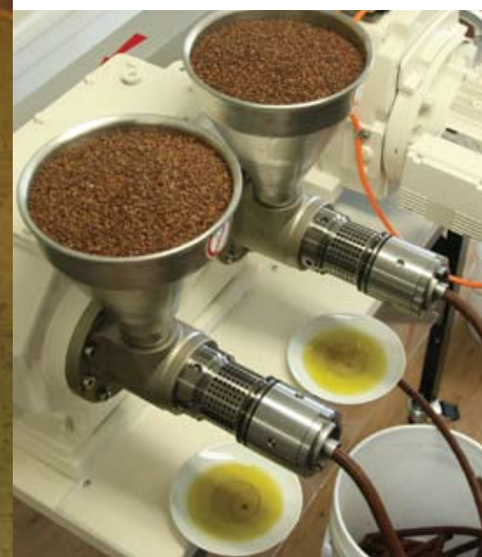
Opposite page: Valentin and Nanette show off a one-ton bag of prepared grape seeds. Below: Grape seeds being milled with the oil flowing into the saucers. The tube of brown “cake” comes out the front. Valentin toasts Dirk Skuras, Managing Director of IBG Monfort, maker of the oil press.
